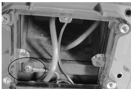
Figure 9.19 - Attach green ground wire
