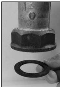
Figure 7.1 - Proper installation of washer into swivel
