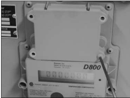
Figure 9.28 - Remove 4 screws on battery cover
