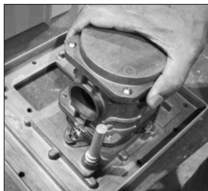
Figure 9.41 - Proper alignment of measurement cartridge
