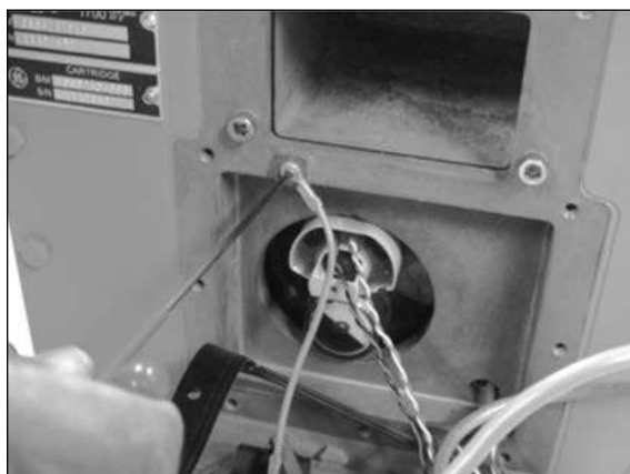
Figure 9.12 - Remove green ground wire
