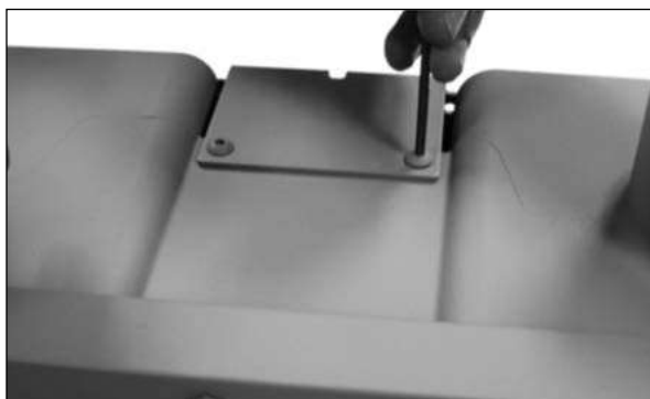
Figure 9.27 - Attach AMR plate to the meter.
