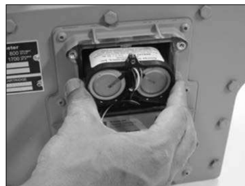
Figure 9.22 - Place battery inside compartment
