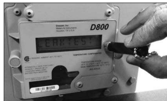
Figure 7.7 - Scroll to LEAKTEST screen
