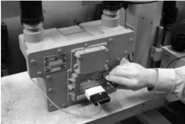
Figure 10.13 - Light on IrDA cable indicates connection is established
