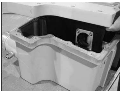
Figure 9.34 - Pull front enclosure off
