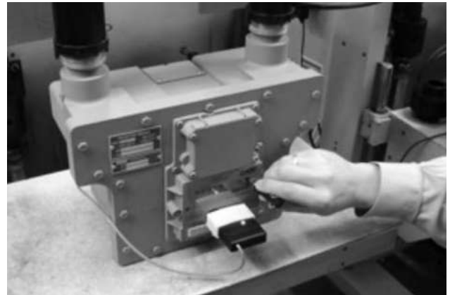
Figure 10.14 - Light on IrDA cable indicates connection is established
