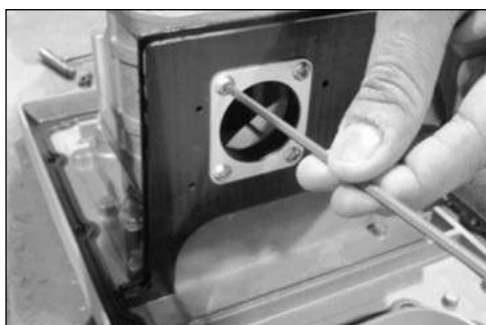
Figure 9.37 - Remove 4 (#10-24) screws on main gasket
