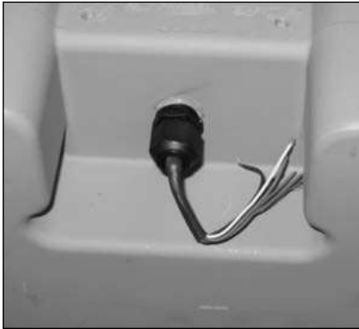
Figure 7.15 - Pulse output cable on backside of meter
