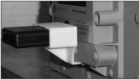
Figure 10.15 - IrDA adapter placed into slot
