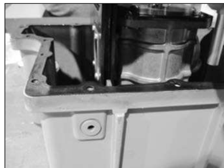
Figure 9.47 - Aligning gasket slots with ribs
