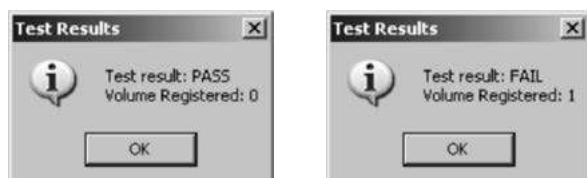
Figure 7.13 - Leak Test Pass/Fail indications in MeterWare
