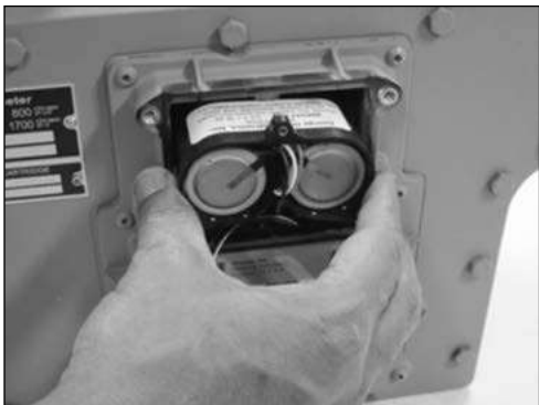
Figure 9.29 - Remove battery pack
