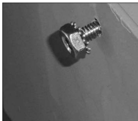
Figure 7.24 - 1/2 screw inserted into top hole of mounting plate
