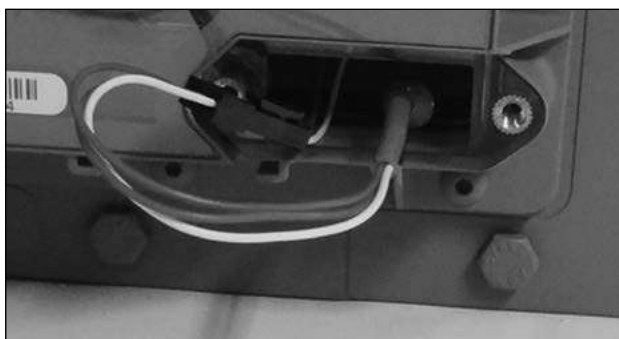
Figure 9.24 - Push temperature probe into probe well
