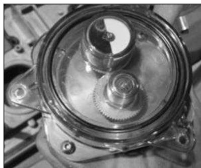
Figure 9.40 - Place O-ring on amber cartridge cover
