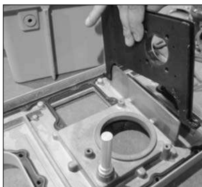
Figure 9.39 - Remove main gasket
