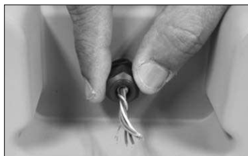
Figure 9.11 - Loosen cable gland connector
