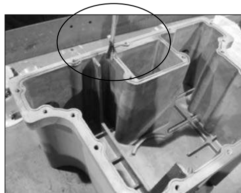
Figure 9.45 - Apply grease to rear enclosure
