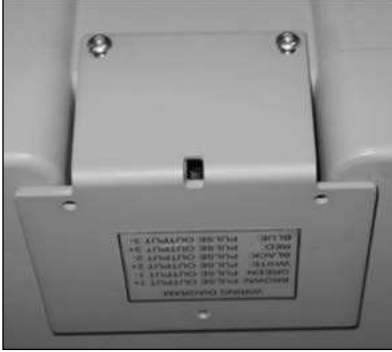
Figure 7.14 - AMR mounting brackets as shipped from factory
