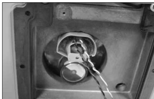
Figure 9.18 - Place Wiegand into compartment
