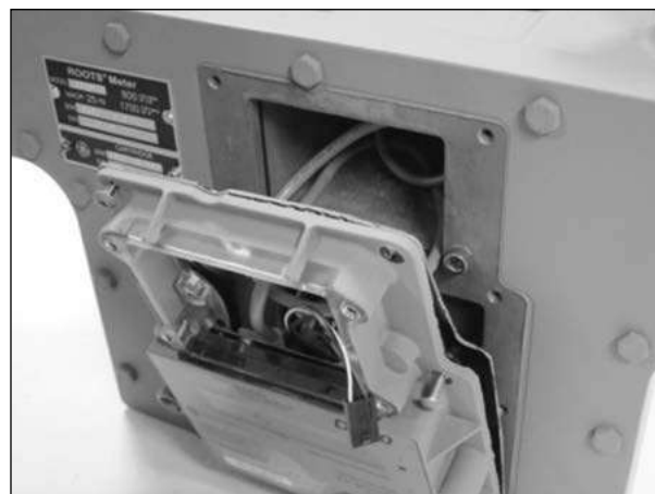
Figure 9.9 - Pull index away from the meter
