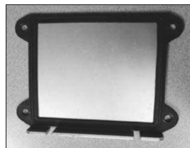
Figure 9.23 - Gasket placed on battery cover
