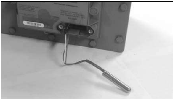
Figure 9.2 - Temperature probe removed from compartment
