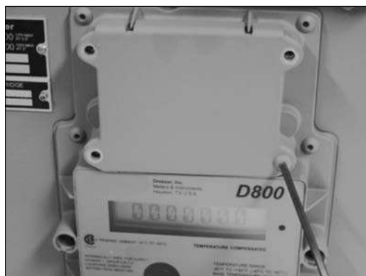
Figure 9.7 - Remove 4 screws on battery compartment
